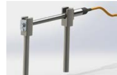
Extensometer (insensitive to temperature)
